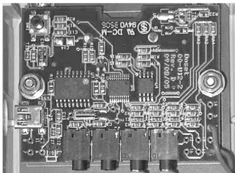
Figure 9: Position of the connection terminals in the OilGuard data logger
