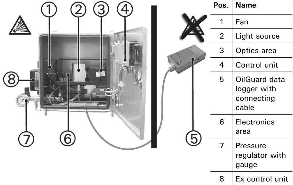
Figure 15: Design of the photometer
