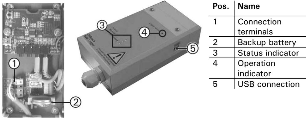
Figure 17: OilGuard data logger
