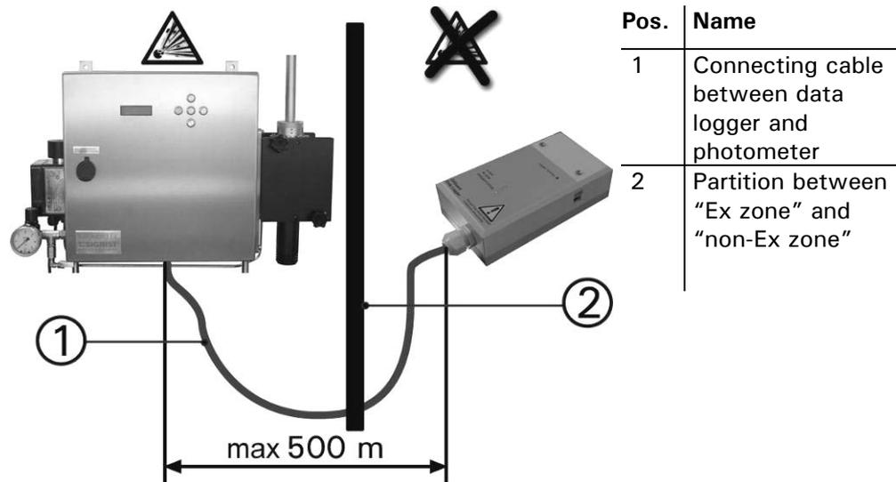
Figure 10: Maximum length of the connecting cable
