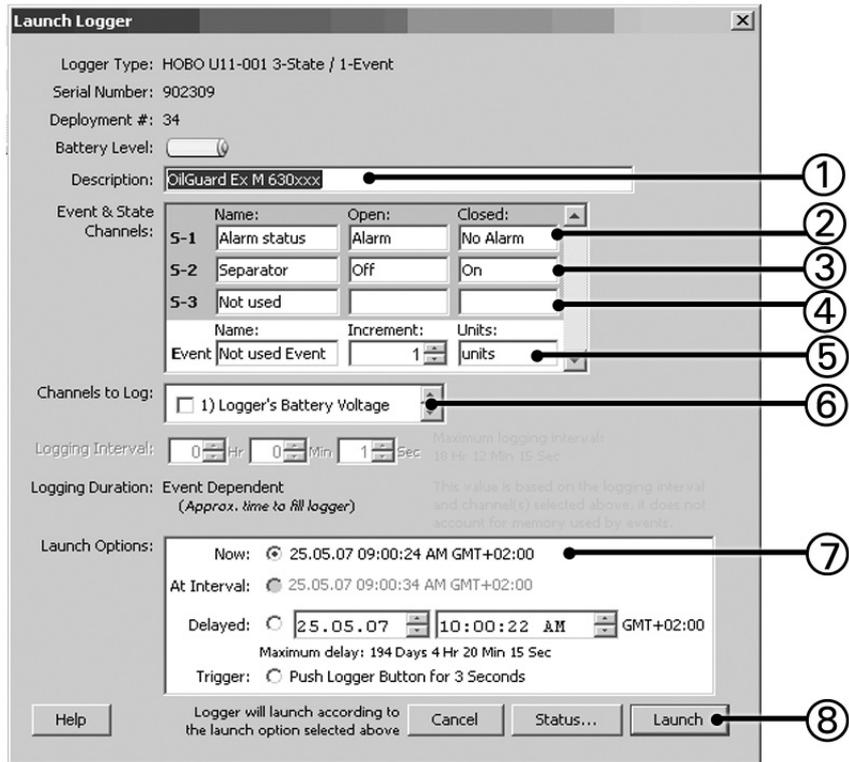
Figure 12 : Check data logger data (HOBOWare)
