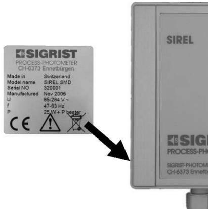
Figure 4 Location of the control unit rating plate
