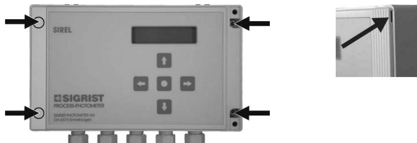
Figure 16: Opening the control unit
