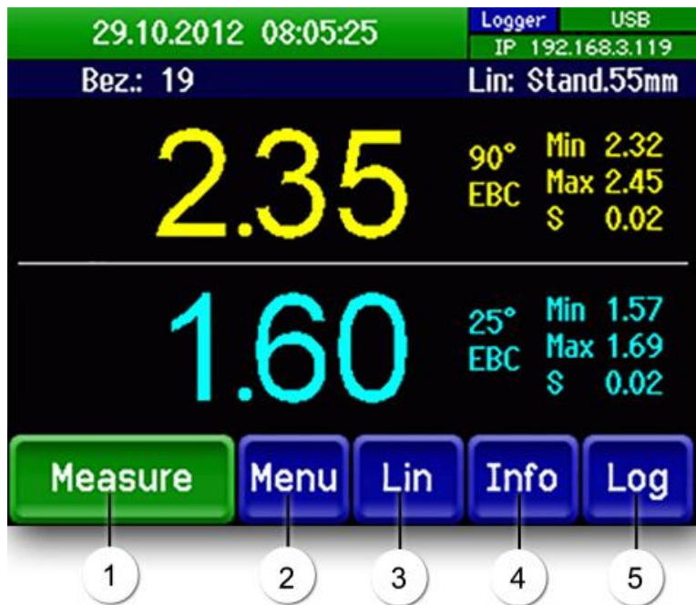
Figure 5: Control elements in normal operation
