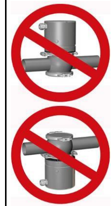
Figure 5: Incorrect mounting position
