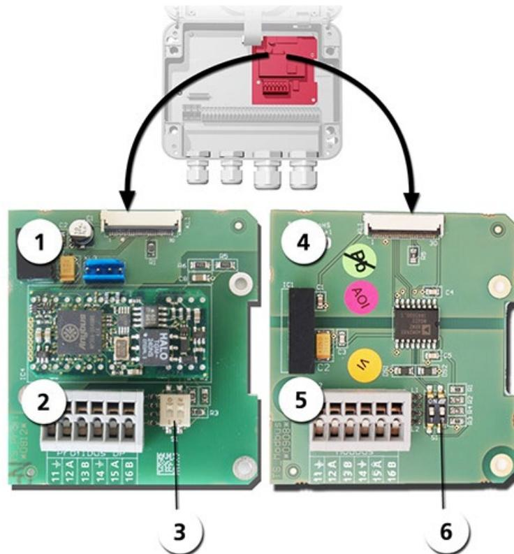
Figure 17: Overview of field bus interfaces
