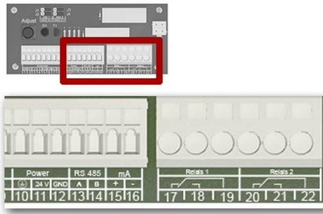
Figure 13: Customer connections on the Conn-R junction box
