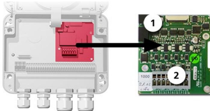
Figure 19: Overview of the 4-way current output module
