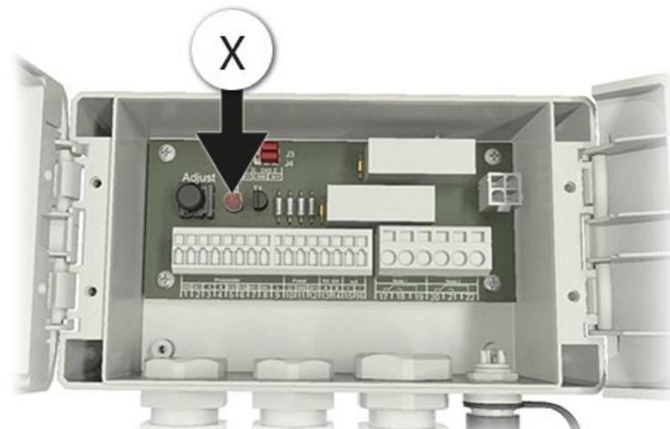
Figure 21: Position of the LED display
