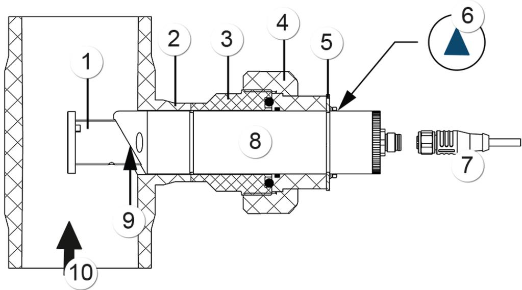
Figure 6: Overview of a measuring point with connection via PE fitting
