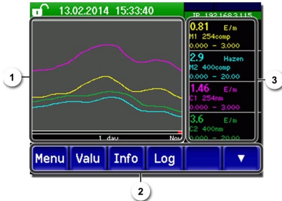
Figure 25: Graphic representation of the measuring values
