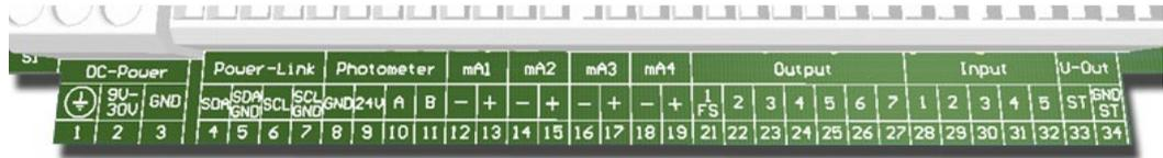
Figure 15: SICON (M) terminal block
