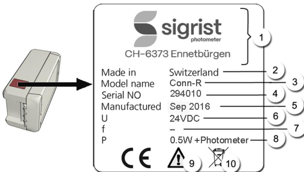
Figure 3: Rating plate on Conn-R junction box
