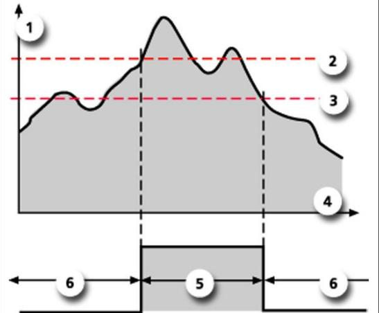
Figure 32: Diagram of limit exceeded
