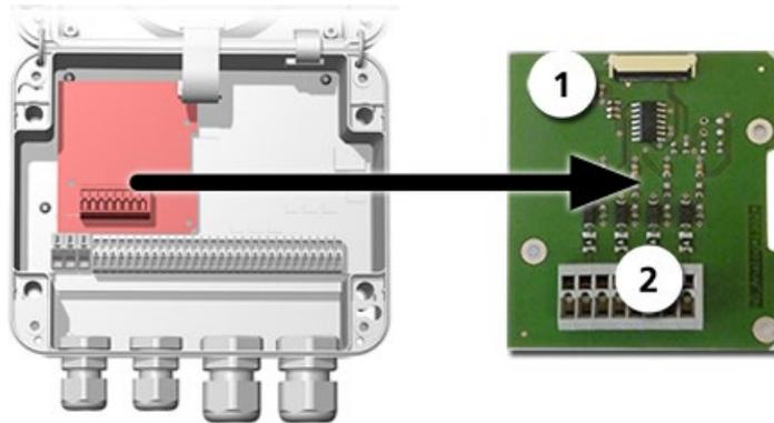
Figure 20: Overview of the 4-way current input module
