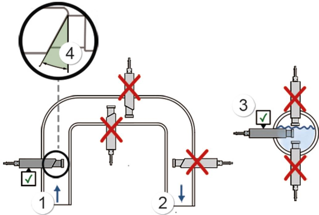
Figure 5: Mounting directions
