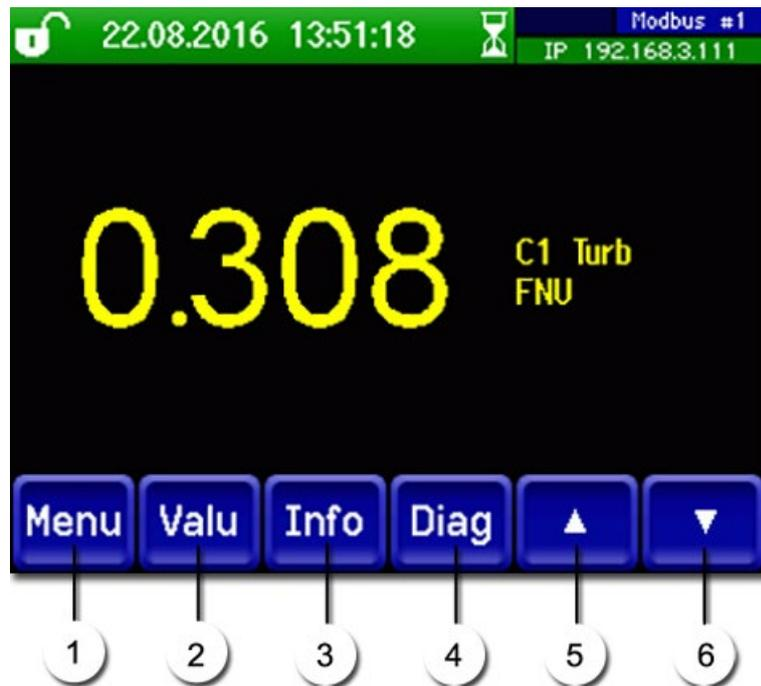
Figure 22: Control elements in measuring operation
