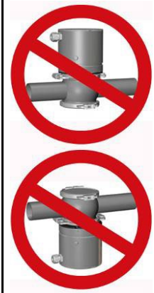
Figure 5: Incorrect mounting position
