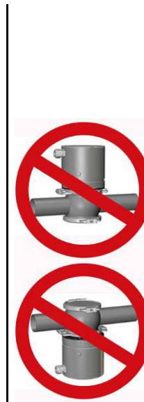
Figure 5: Incorrect mounting position
