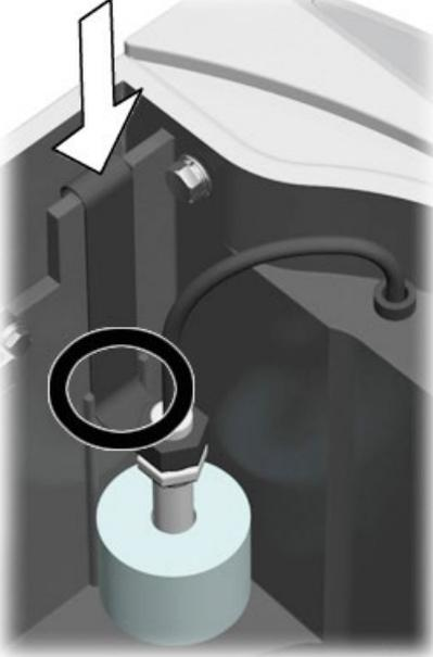
A close-up diagram of the float mechanism. A white arrow points down to a circular track (glissière) on the lid. A black circle highlights the float mechanism, which is shown as a light blue cylindrical component with a black ring on top, positioned within the track.      |
