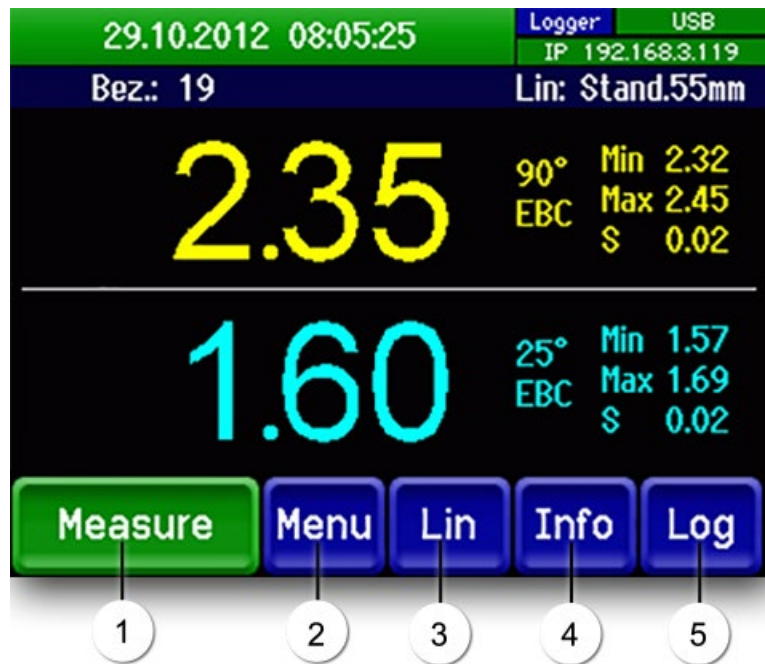
Figure 5: Control elements in normal operation
