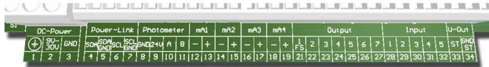
Figure 19: SICON (M) terminal block
