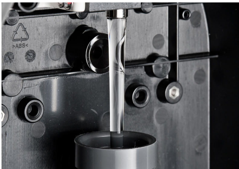
Contactless measurement of the free-falling water jet – guaranteed pollution-free.
