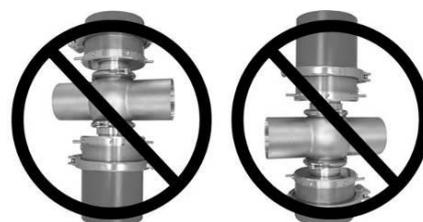
Figure 9: Installation in horizontal product pipes.
