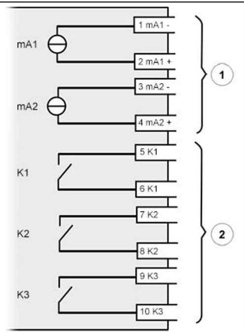
Figure 1: Outputs diagram
