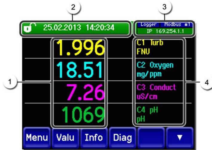
Figure 21: Displays in measuring mode
