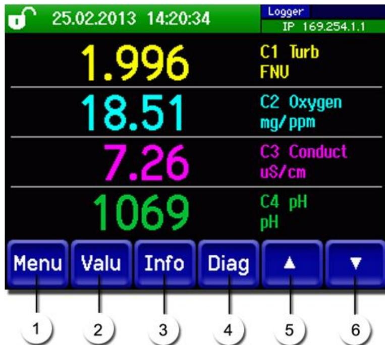
Figure 15: Control elements in measuring mode
