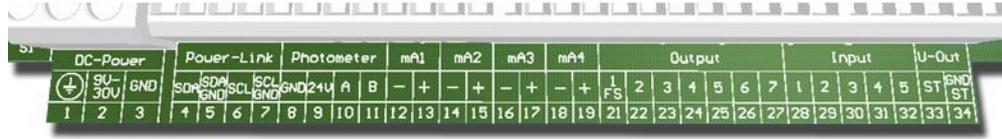
Figure 6: SICON M terminal block
