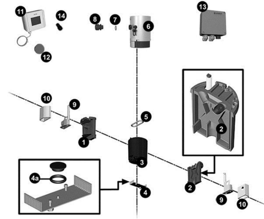
Please fold out
