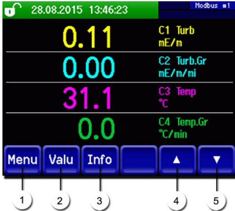
Figure 12: Control elements in measuring operation
