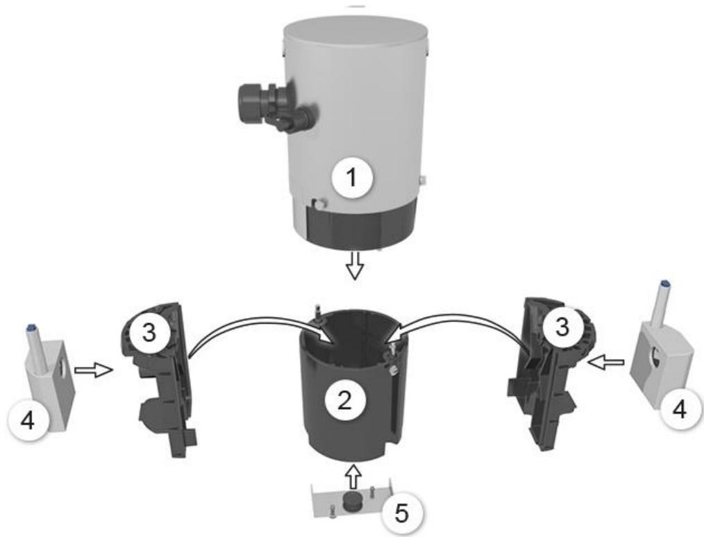
Figure 23: Exploded drawing of the FireGuard 2 Integral
