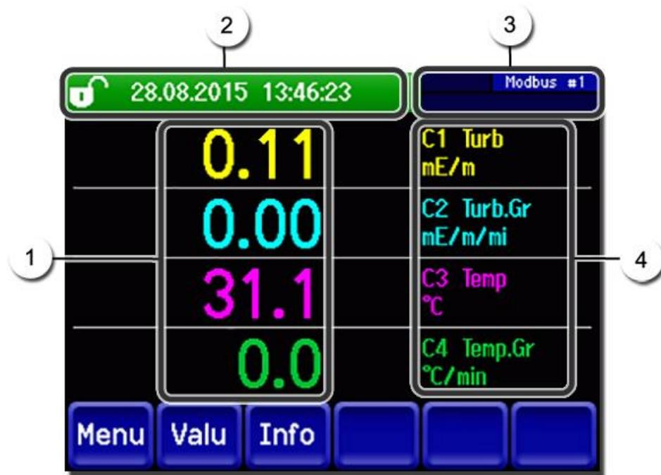
Figure 15: Display in measuring operation
