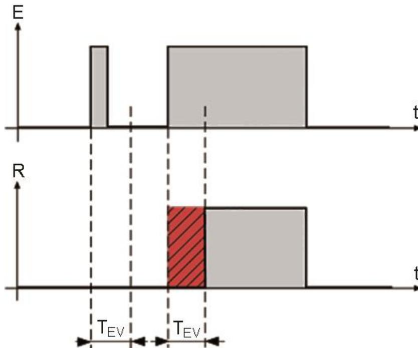
Figure 20: Cut-in delay
