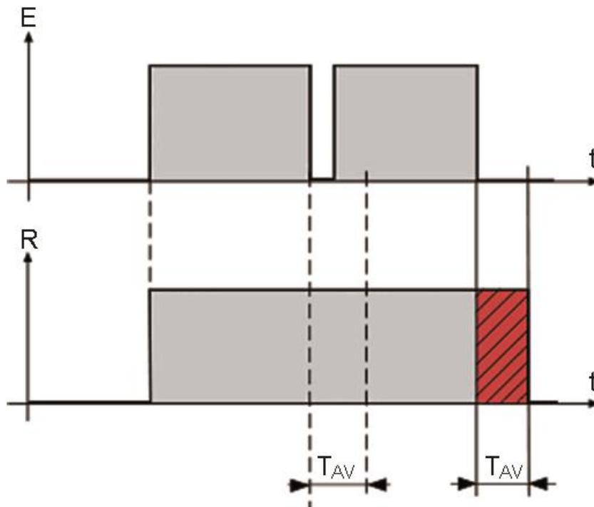
Figure 21: Cut-out delay
