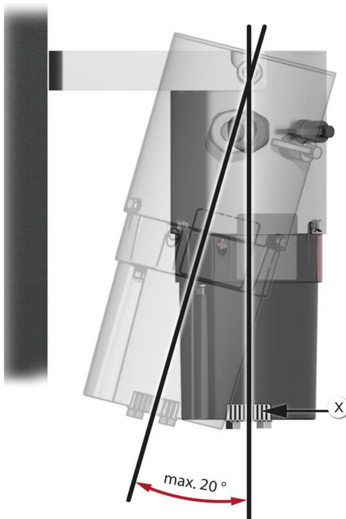
Figure 5: Installation position in the air flow
