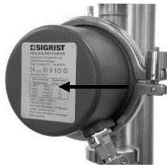
Figure 4: Photometer rating plate.
