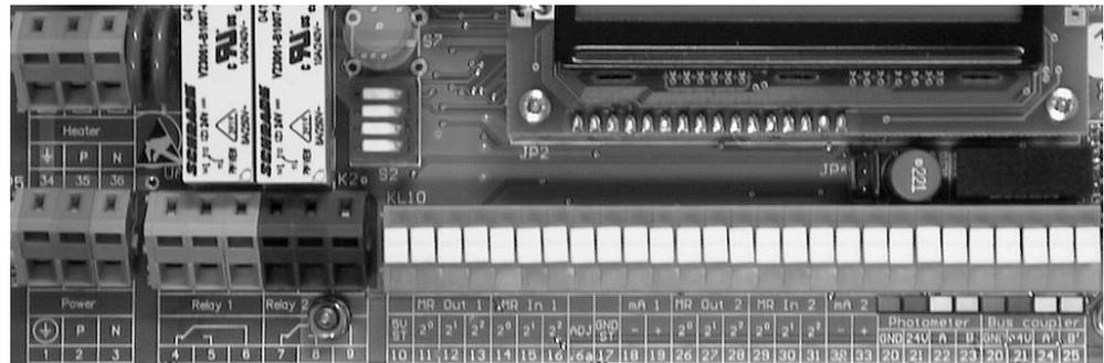
Figure 11: Terminal block for SIREL SMD 100..240 VAC.
