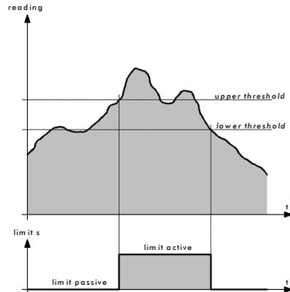
Figure 15: Upper and lower thresholds of a limit.
