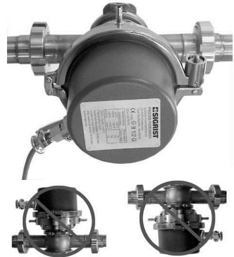
Figure 7: Installation in horizontal product pipes.
