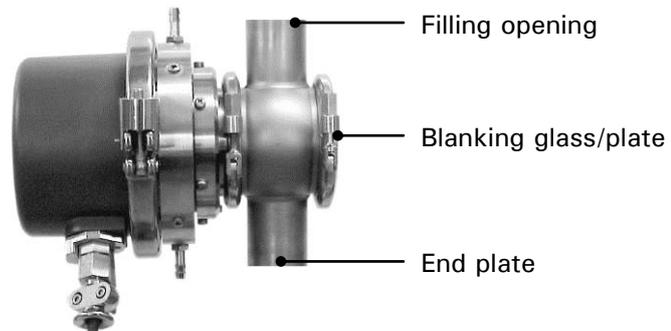
Figure 17: Test setup for formazine recalibration.
