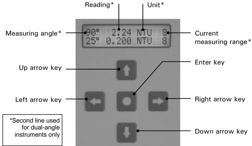
Figure 12: Operating elements and display.
