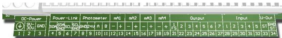
Figure 6: Bornier SICON (M)
