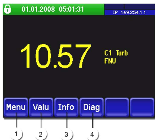
Figure 1: Control components in normal operation
